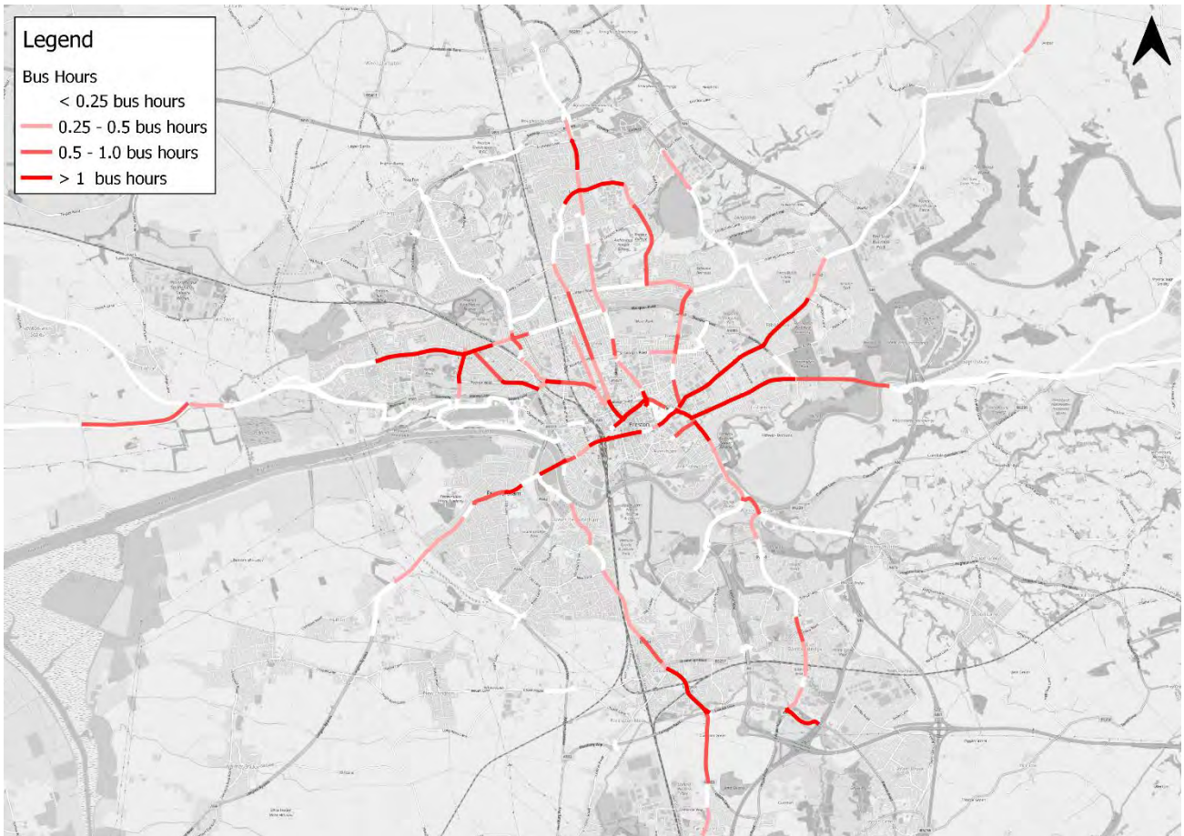
Figure 2-9: delays to buses due to congestion across the City Region in bus vehicle hours lost across an average weekday
